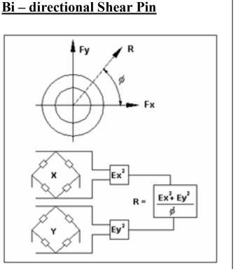
When both magnitude & directional force are unknown these can be measured with Bi – directional shear pin.
